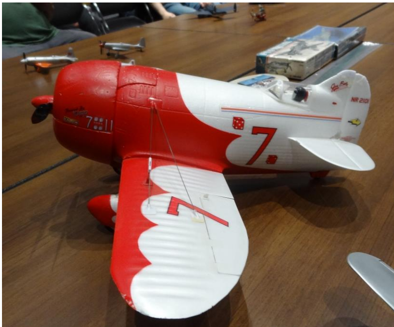
Dave Balderrama's 1:12 scale GB Super Sport is actually a flying model, with an electric motor under the cowling. It's made of styrofoam, and the top of the vertical fin attests to how durable it is!
